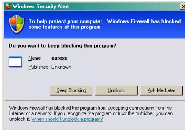
With the Windows Firewall, the user may choose to unblock the Earexe executable from the security alert dialog above. However, if you are operating across a cluster, this will not be sufficient to enable Parallel Phoenix to run. There are additional settings needed on both the master and slave PCs.
